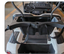
Storage basket with cable tie
